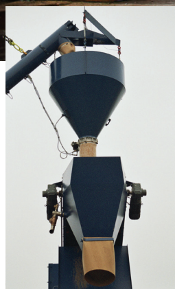
Cement weighing and delivery chute
