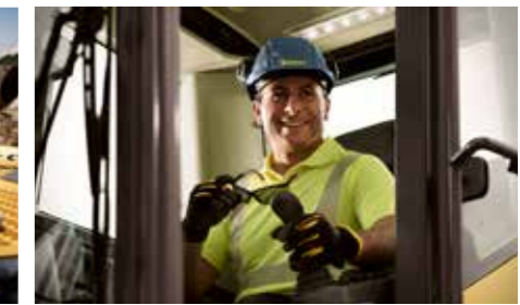
The quiet, air-conditioned safety cabin is ROPS and FOPS-approved. A happy operator means better productivity.
