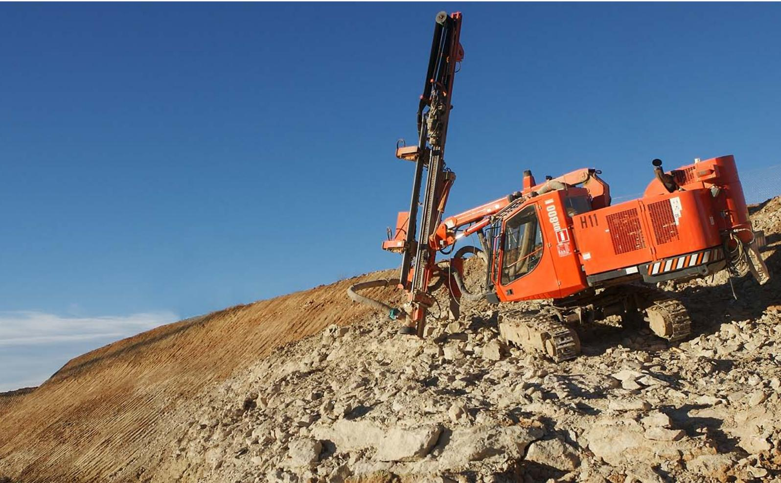
Sandvik DX800 is a hydraulic, self-propelled, self-contained, crawler based surface drilling rig equipped with a cabin (F.O.P.S. and R.O.P.S.) and rod handling system.
